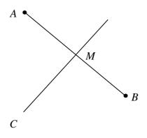
Line CM is drawn perpendicular to AB using a set square or a pair of compasses and ruler.
