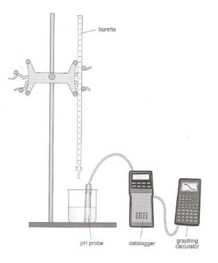
If a datalogger is not available the measurements made using a pH meter or conductivity meter can be logged by recording the measurements in table format using pen and paper.
